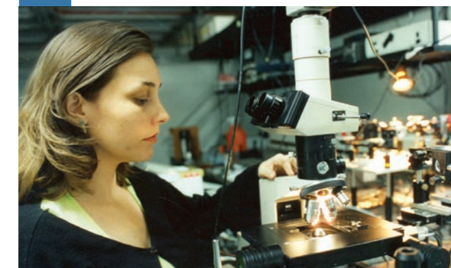
Confocal laser scanning biological microscope at the biophotonics lab
